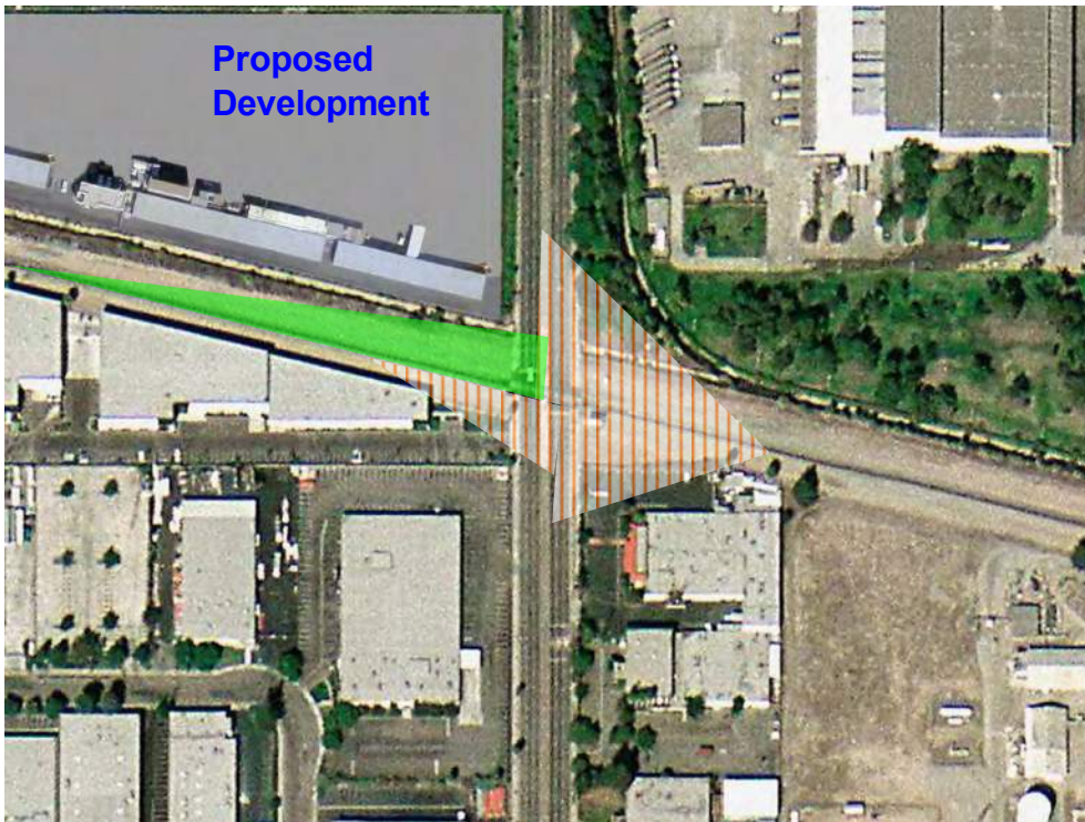
Figure 3-17. Sight Triangle Impeded by Adjacent Buildings
