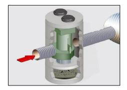
Figure 2: Hydrodynamic Separator Schematic
