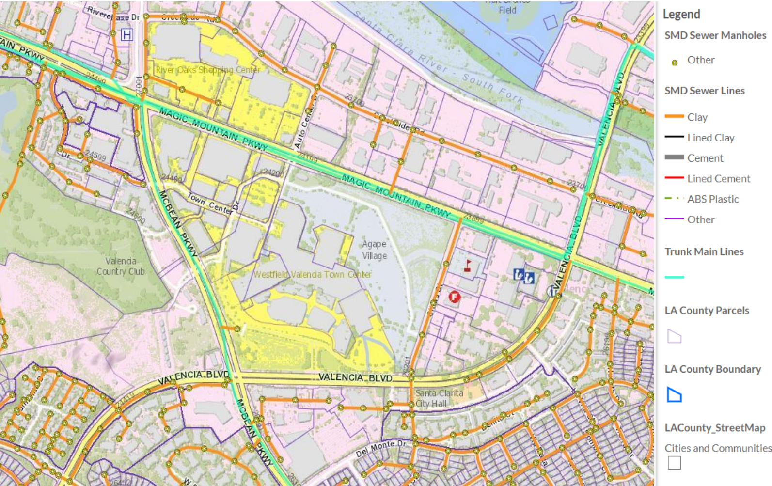
Figure 3-6. Existing SMD Sanitary Sewer Facilities
