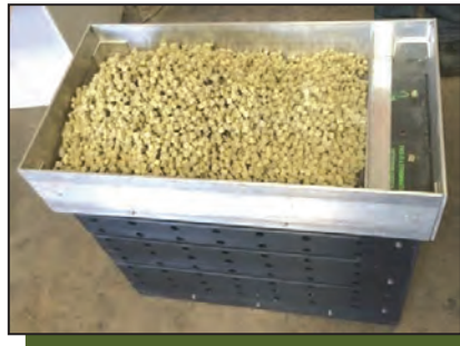
Refilling tray on cartridge with bulk media.
