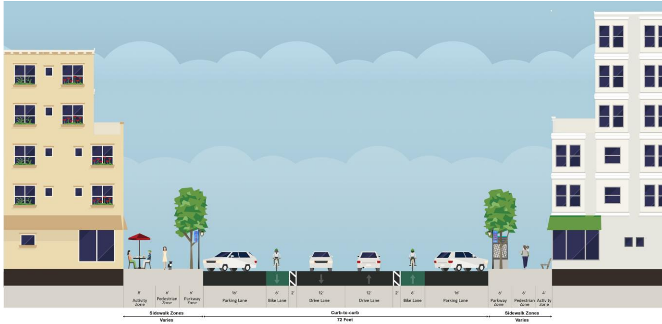
Figure 2-21. Cross-Section of Major Connector with Angled Parking
