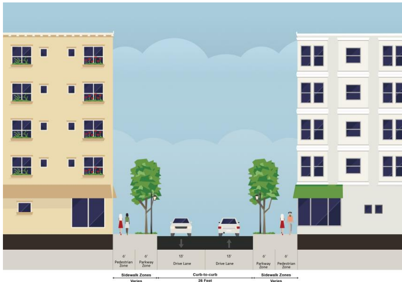
Figure 2-26. Cross-Section of Type B Internal Road
