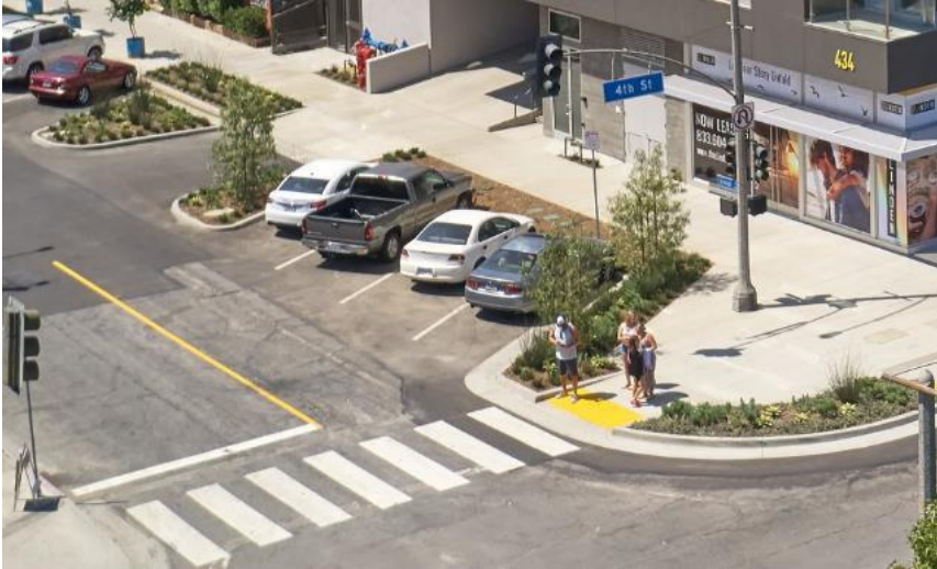
Figure 2-47. Example of Parking with Bulb-outs
