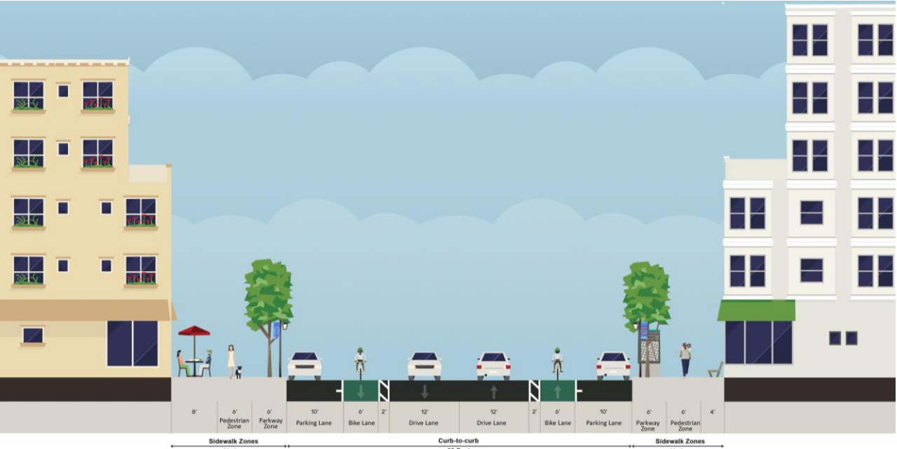
Figure 2-23. Cross-Section of Major Connector with Parallel Parking
