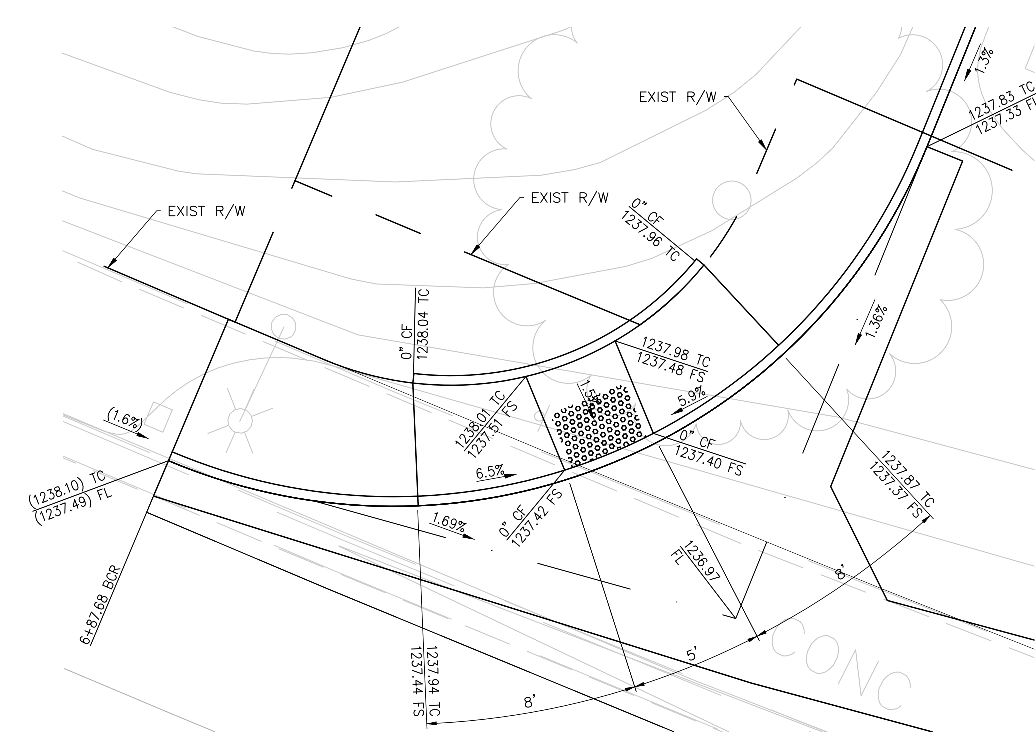
CURB RAMP NW CORNER PROPOSED ENTRANCE SCALE: 1"=5'
