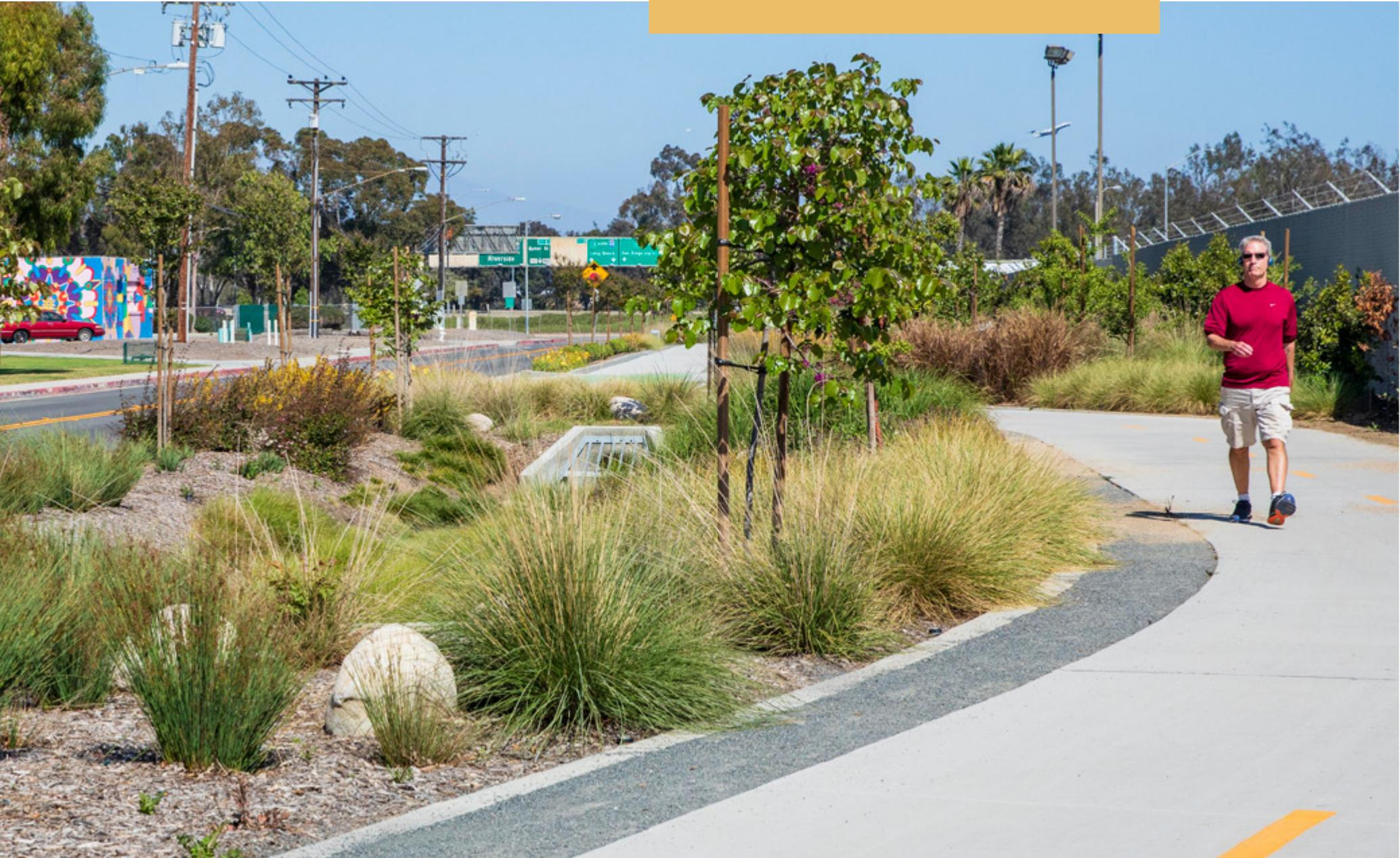
*Curb side vegetated swale with meandering walking/biking trail*
