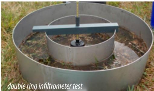
double ring infiltrometer test
