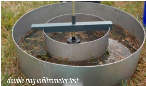
*double ring infiltrometer test*
