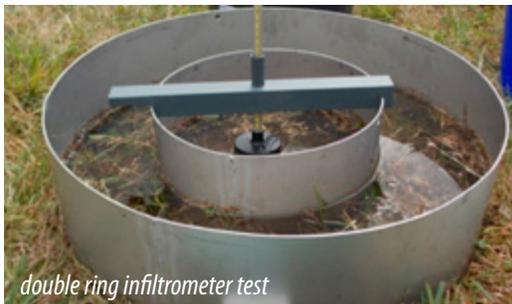
double ring infiltrometer test
