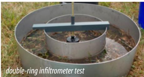
*double-ring infiltrometer test*
