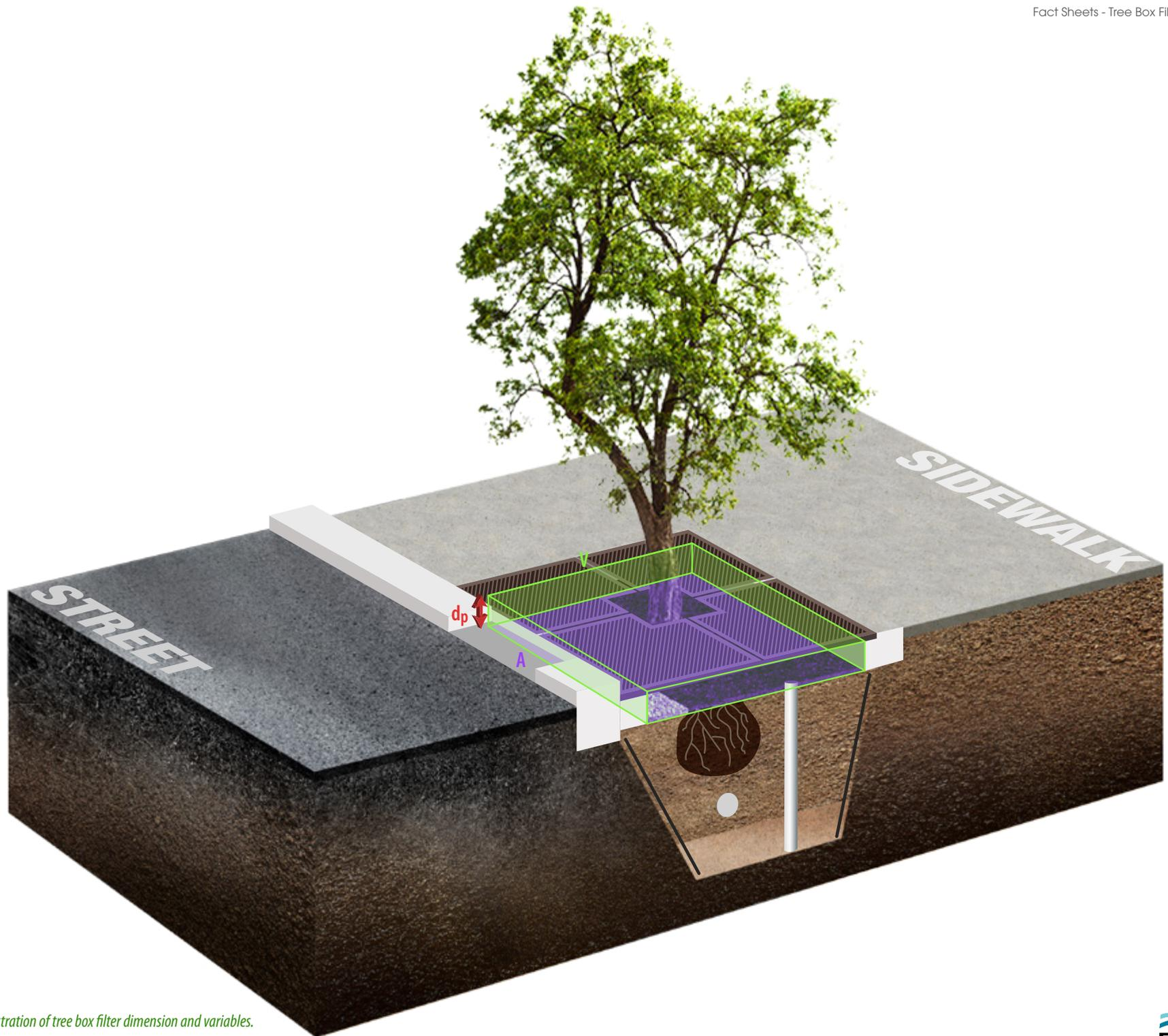
*Isometric illustration of tree box filter dimension and variables.*
