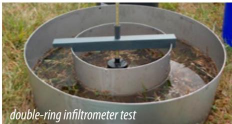
*double-ring infiltrometer test*
