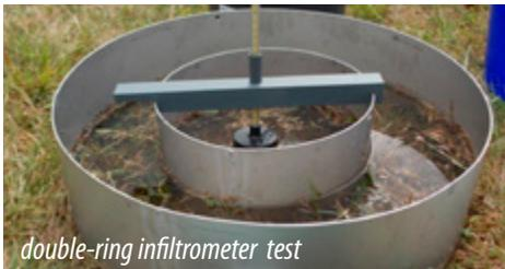
*double-ring infiltrometer test*
