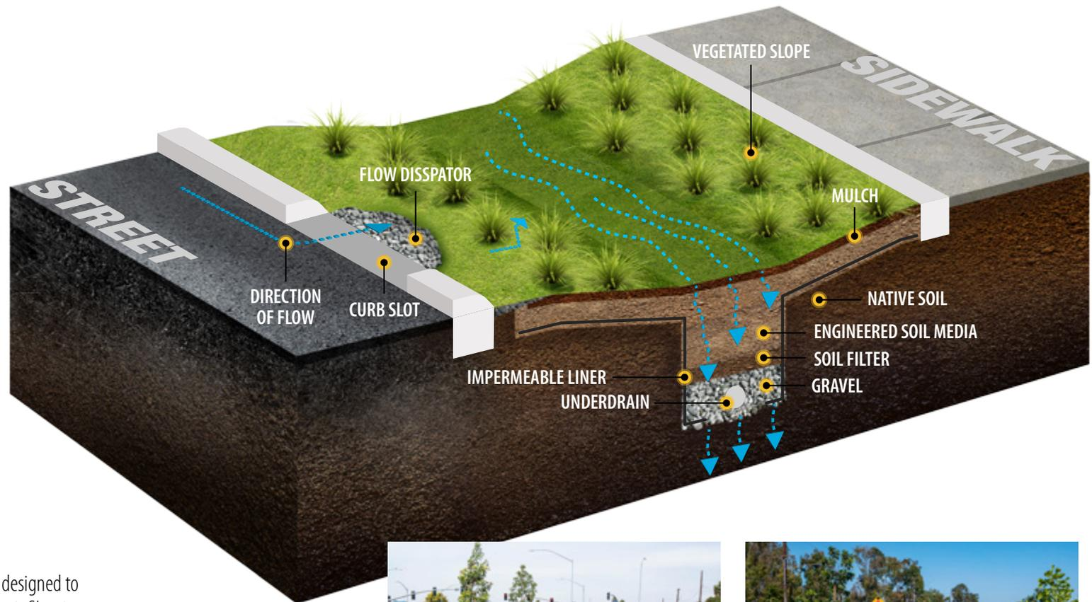
Specialized vegetated channels designed to slow stormwater runoff, promote infiltration, trap sediment, and treat pollutants.
