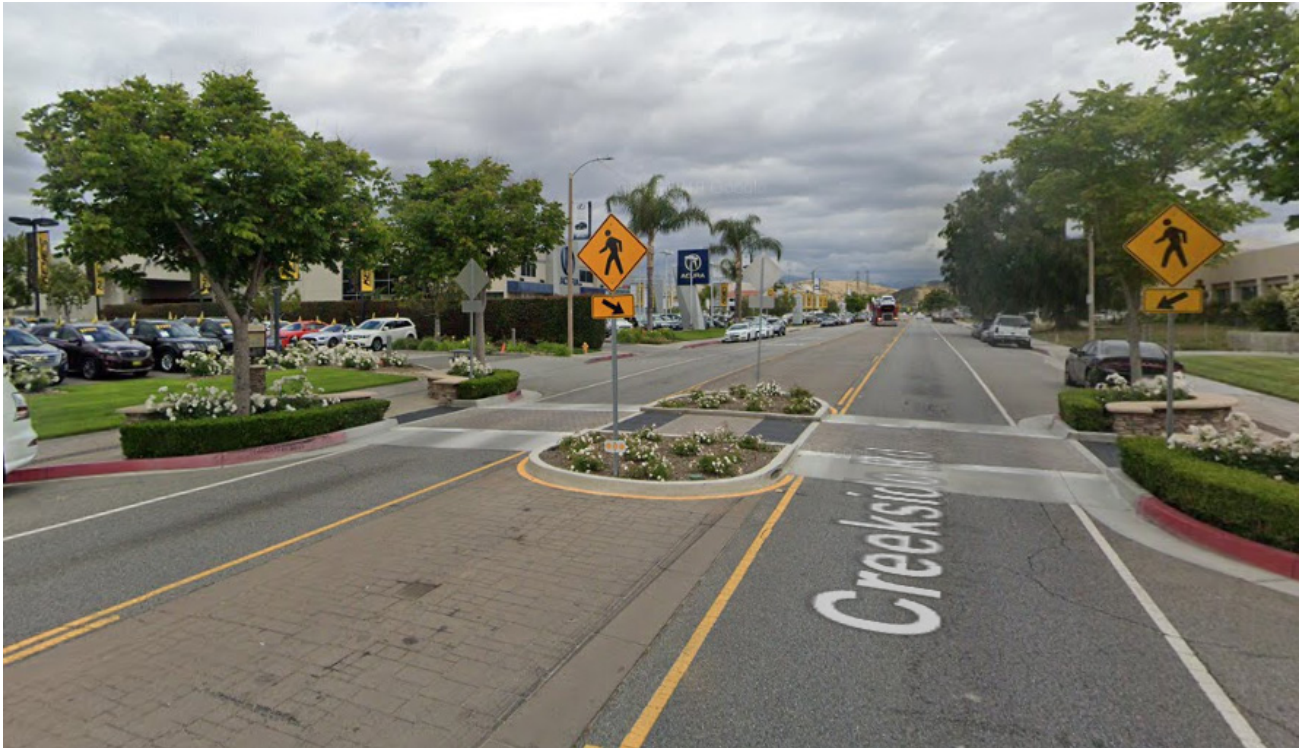
Mid-block crossings on Creekside Road include pedestrian refuges, bulb-outs, raised tables, and landscaping. (Google Streetview)
