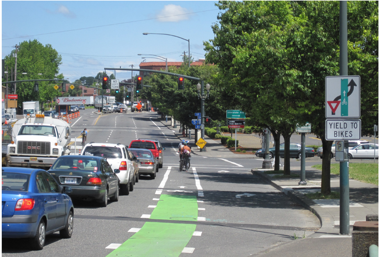
Below: Green conflict striping helps alert bicyclists that drivers might be crossing the bicycle lane, and drivers that bicyclists have the right of way.
