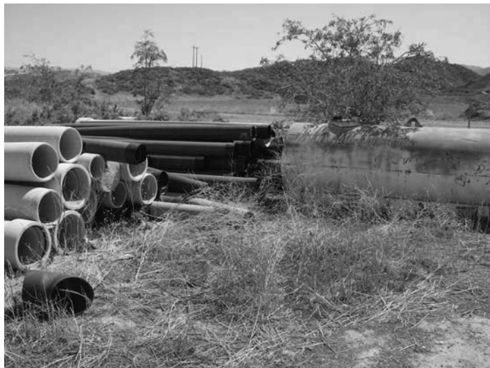
Transite Pipe Storage and Empty Fuel Tank in SE Corner
